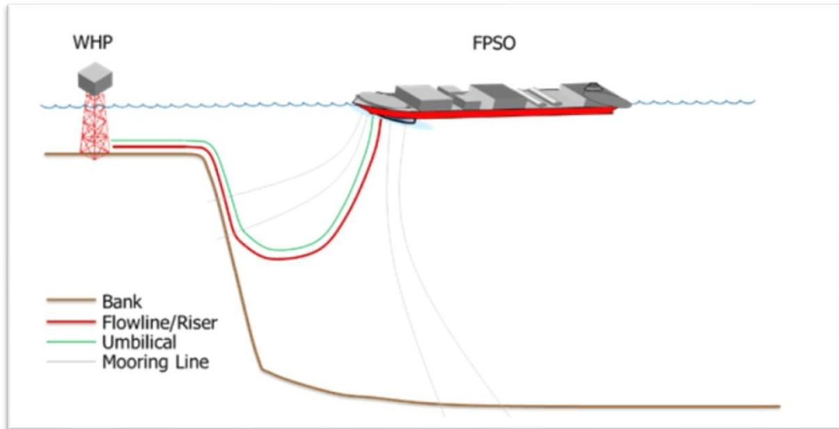
Figure 1: Buffalo Field Layout Schematic
