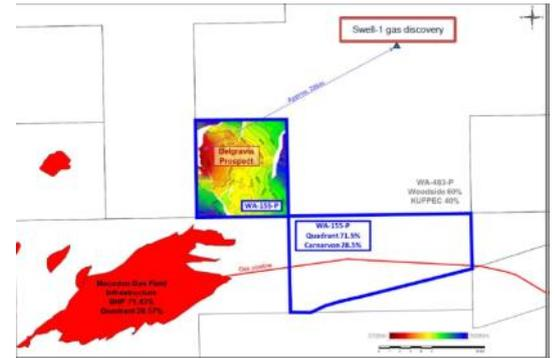
Carnarvon's mapping indicates the crest of the Belgravia structure is up-dip of the Swell gas discovery and around 650 metres shallower than the Swell-1 structure. Carnarvon expects that the Belgravia target could contain better reservoir quality compared to that reported at Swell.
