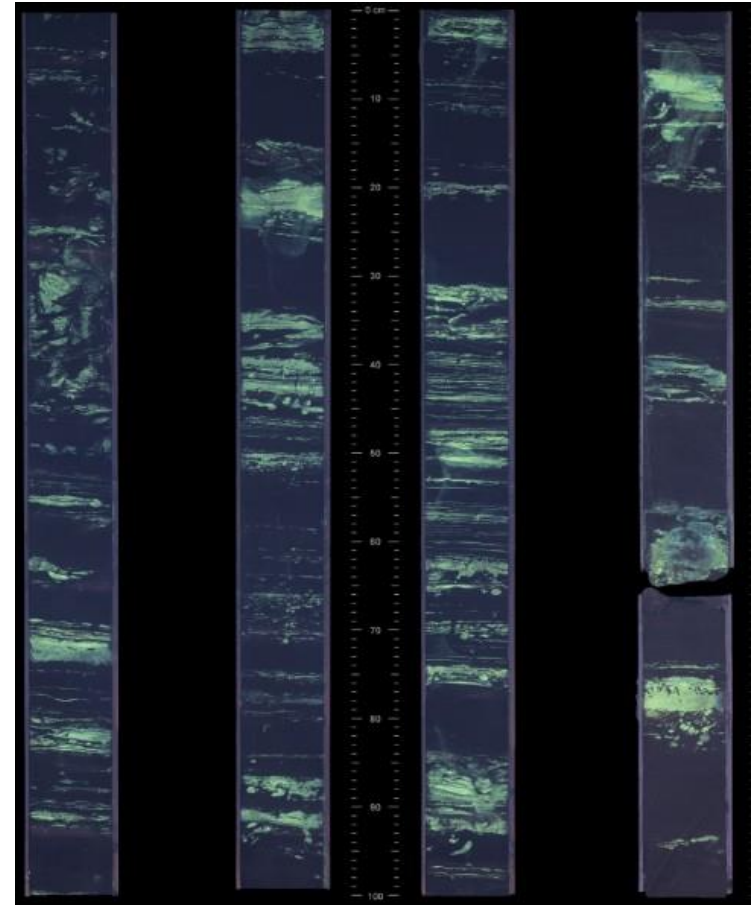
Preliminary ultraviolet light photographs of the Outtrim East-1 core outlining hydrocarbon occurrences in the reservoir
