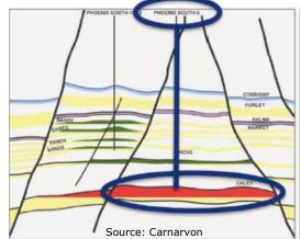
Small volumes of associated gas at the Phoenix South location will lower operating cost by providing free fuel for an FPSO operating on an oil discovery.
