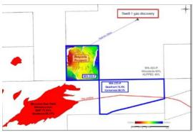
Carnarvon's mapping indicates the crest of the Belgravia structure is up-dip of the Swell gas discovery and around 650 metres shallower than the Swell-1 structure. Carnarvon expects that the Belgravia target could contain better reservoir quality compared to that reported at Swell.
